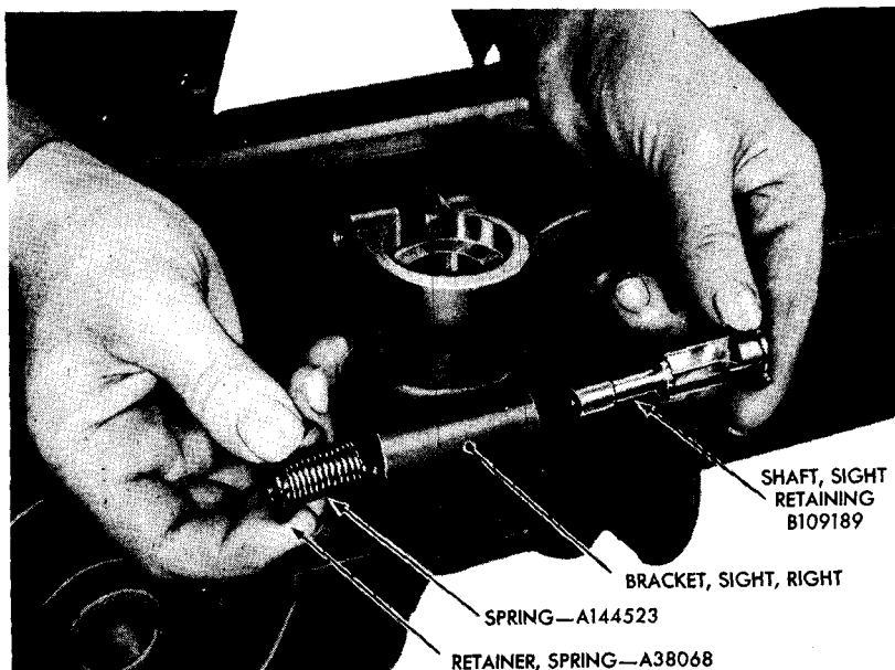
Figure 56 — Removing Sight Retaining Shaft and Spring
