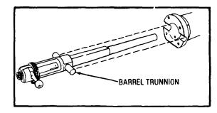
Step 5: Place the gun barrel in the adapter and engage the barrel trunnions with the adapter slots.
