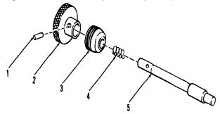
DRILL HOLE FOR SPRING PIN (1) IN REPLACEMENT KNOB (2) OR PLUNGER (5) AS FOLLOWS:
