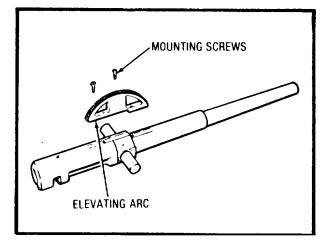
**Step 6:** Remove the elevating arc from the gun barrel by removing the two mounting screws.
