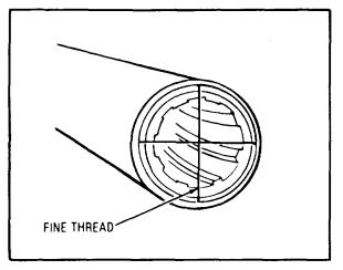
**Step 4:** Attach fine thread across the four witness marks on the end of the tube by using a rubber band. Also place boresight strings on the muzzle of the howitzer
