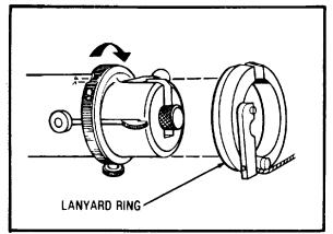
**Step 13:** Turn the safety ring to the "fire" position. Place the lanyard ring over the rear of the breech, matching the openings of breech and the lanyard ring.
