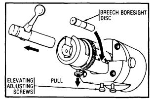
**Step 11:** Lock the barrel into position by securing the adapter cap to the body. Small bolt goes in upper right hole. Do not tighten the four screws yet.
