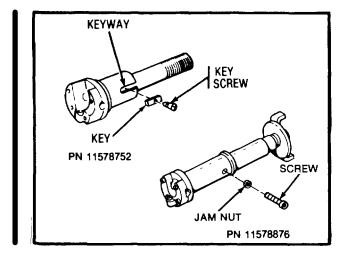
**Step 4:** Install the key in the keyway and secure with a screw.
