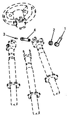
TIGHTEN REPLACEMENT SCREW (4) FINGER TIGHT WITH LEVER (1) IN THE 3 O'CLOCK POSITION, THEN DRILL AND TAP HOLE FOR SETSCREW (3). AR 902766
