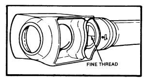
**Step 7:** Attach fine thread across the tour witness marks on the end of the tube by using a rubber band. Also place boresight strings on the muzzle of the howitzer.
