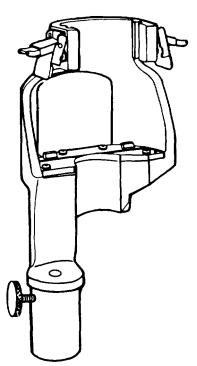
TELESCOPE SUPPORT ASSEMBLY (PN 11728907) For M117 Panoramic Telescope
