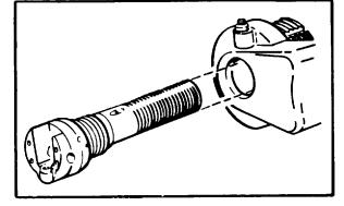
Step 5: Insert the adapter (top up) in the breech-block.
