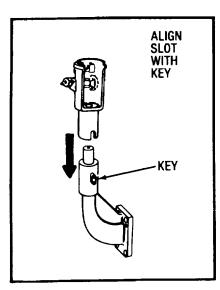
**Step 7:** Attach the telescope socket, holder, or support assembly to the mount assembly.
