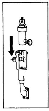
**Step 9:** Place the panoramic telescope into the telescope socket, holder, or support assembly.
