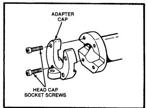
**Step 5:** Remove the four head cap socket screws and the adapter cap.
