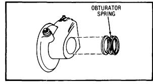
**Step 3:** Place the obturator spring in the firing mechanism housing recess.
