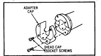
Step 7: Remove the four head cap socket screws and the adapter cap.
