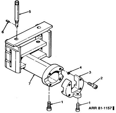
Figure C-22A. Adapter assembly for M102 - optional manufacture
