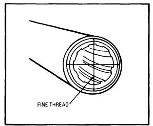
Step 4: Attach fine thread across the four witness marks on the end of the tube by using a rubber band. Also place boresight strings on the muzzle of the bowitzer.
