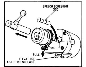
**Step 12:** Close the breech, remove the bolt by pulling down on the locking cap and pulling bolt to the rear. To boresight the 14.5 mm device:
