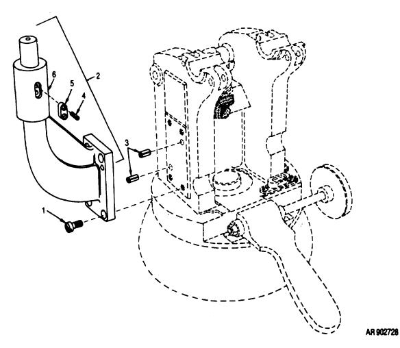
Figure C-7. Telescope bracket removed from mount
