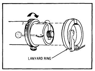
**Step 8:** Turn the safety ring to the "tire" position. Place the lanyard ring over the rear of the breech, matching the openings of breech and the lanyard ring.
