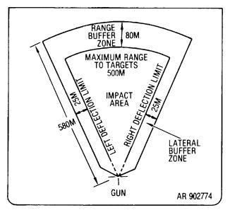
Figure 2-3. Example of computed surface danger zone
