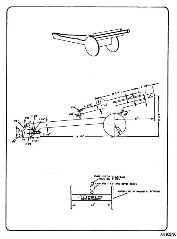
Figure 2-9. 105-mm Howitzer target model
