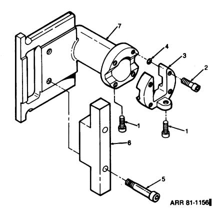
Figure C-21A. Adapter assembly for M101A1 - optional manufacture
