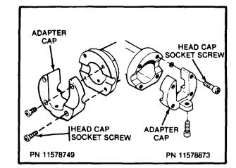
Step 2: Remove the four head cap socket screws and the adapter cap.
