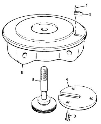
DRILL 0.118 + 0.004 DIAMETER HOLES FOR SPRING PINS (1) IN REPLACEMENT KEY (2). PINS MUST BE FLUSH WITH TOP OF KEY.
