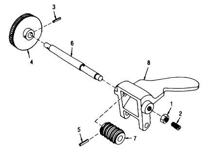
PRESS WORM GEAR AND HANDWHEEL TIGHT AGAINST SHOULDER AND DRILL 0.078 + 0.004 TO ACCEPT SPRING PINS (3 AND 5)
