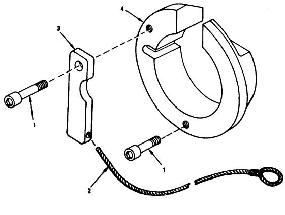
AR 902739 Figure C-25. Lanyard ring assembly, 14.5mm gun - exploded view
