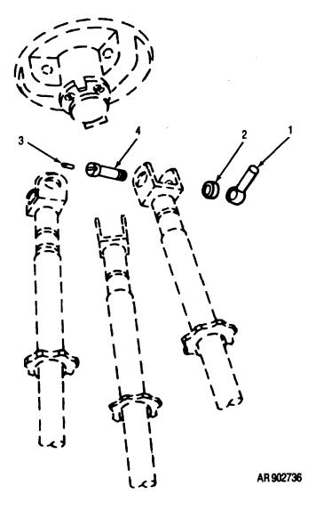
Figure C-14. Tripod locking lever group - exploded view
