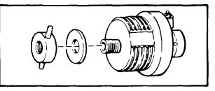
**Step 6:** Place the washer on the adapter. Tighten the nut all the way down, then loosen it two turns. The loosening of the nut allows the breech to be closed fully.
