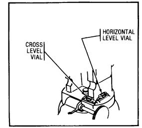
**Step 1:** Center both the horizontal and the cross level vial bubbles.
