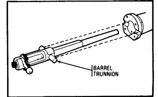
**Step 10:** Place the gun barrel in the adapter and engage the barrel trunnions with the adapter slots.
