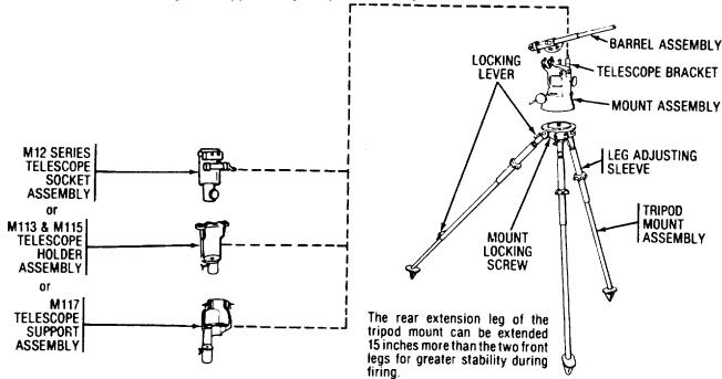
Figure 1-1. Mount and tripod assemblies.
