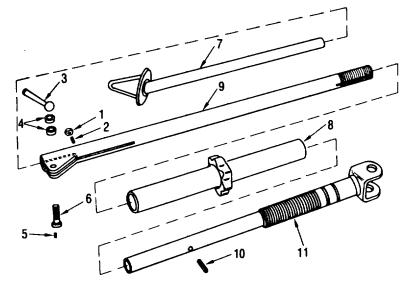
DRILL AND TAP HOLE FOR SETSCREW (5) IN SCREW (6) AT ASSEMBLY.
