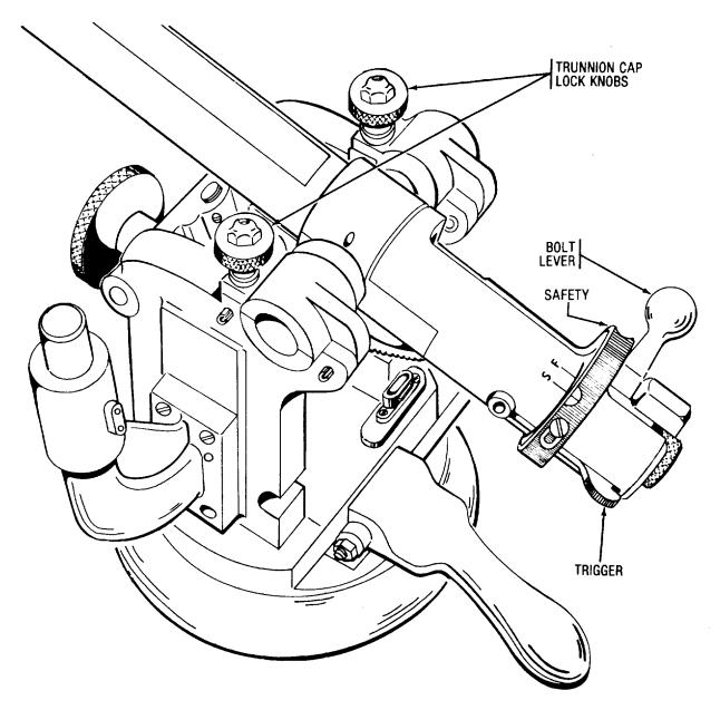
Figure 1-3. Barrel assembly.
