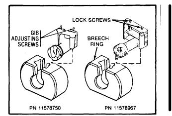
**Step 1:** Open the breech and place the adapter in the breech recess. The gib adjusting screws should be in the unscrewed position. Make sure the adapter rests against the breech ring then turn the gib screws finger tight. Tighten the screws an additional 1/2 turn. Loosen lock screws before positioning adapter PN 11578967 in breech recess. Tighten the screws to lock adapter in breech ring.
