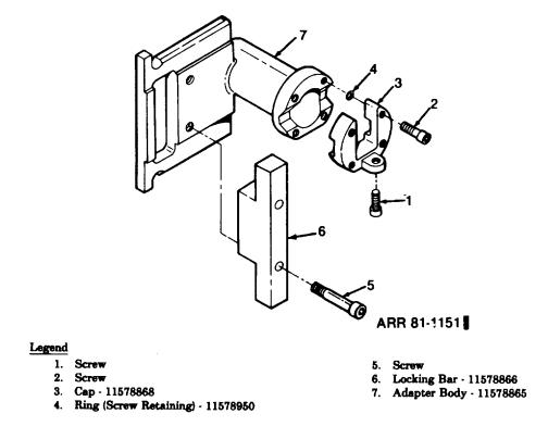
Figure 4-5A. Disassembly/assembly of adapter assembly PN 11578873 for M101A1
