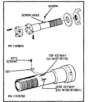
**Step 3:** Install the key in the appropriate keyway and secure with a screw: The top keyway is for the M107/M110 weapons, the side keyway is for the M109 and M109A1 155-mm howitzers. Adapter PN 11578870 has no keyway. Install screw in appropriate screw hole.
