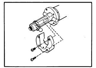
**Step 11.** Lock the barrel into position by securing the adapter cap to the body (short screw in upper right hole). Do not tighten the four screws yet.
