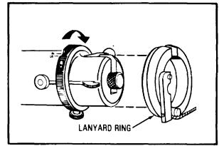
**Step 13:** Turn the safety ring to the "fire" position. Place the lanyard ring over the rear of the breech, matching the openings of breech and the lanyard ring.
