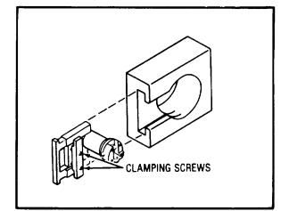
**Step 1:** Open the breech and place the adapter in the breech recess. (If the weapon is going to be moved, remove the breech block). Make sure the two clamping screws are in an unscrewed position. Tighten the two clamping screws.
