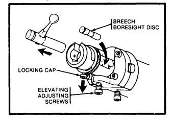
**Step 10:** Close the breech, remove the bolt by pulling down on the locking cap and pulling bolt to the rear. To boresight the 14.5-mm device:
