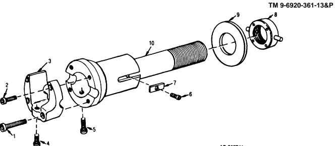
AR 902741 Figure C-23. Adapter assembly for M 14 and MII4AI - exploded view
