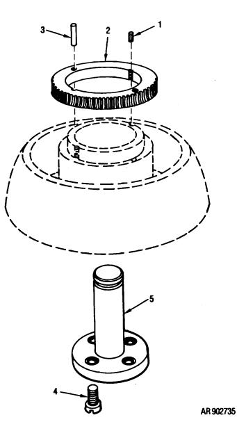
Figure C-13. Fixed mount base assembly - exploded view
