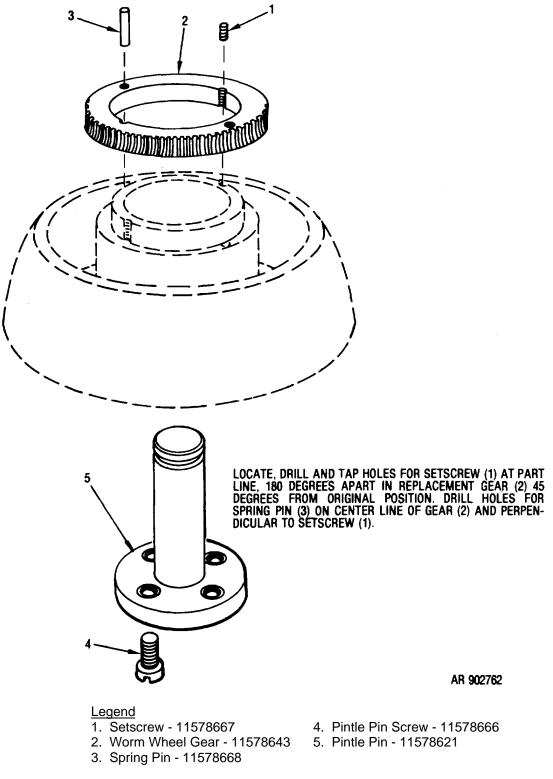
Figure 6-9. Disassembly/assembly of fixed mount base assembly
