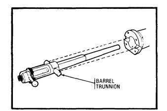
**Step 8:** Place the gun barrel in the adapter and engage the barrel trunnions with the adapter slots.
