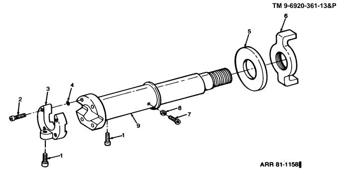
Figure C-23A. Adapter assembly for M114A - optional manufacture
