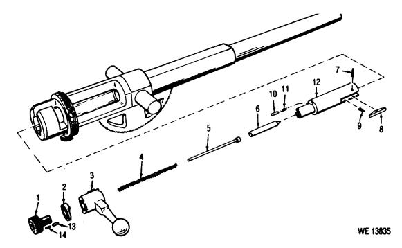
Figure C-4. Breechbolt group - exploded view
