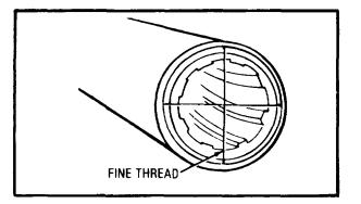
**Step 9:** Attach fine thread across the four witness marks on the end of the tube by using a rubber band. Also place boresight strings on the muzzle of the howitzer.
