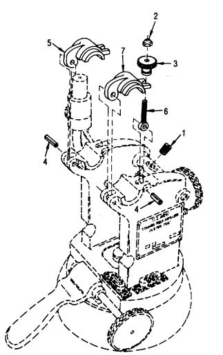
FILE CONCAVE SURFACE OR REPLACEMENT TRUNNION CAPS UNTIL CANNON WILL ELEVATE AND DEPRESS WITHOUT BINDING.
