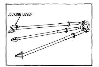
**Step 1:** Remove the tripod assembly from the storage chest. (Note that the rear leg has the locking lever near the bottom).
