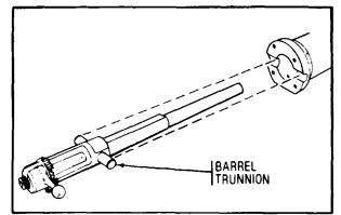
**Step 5:** Place the gun barrel in the adapter and engage the barrel trunnions with the adapter slots.
