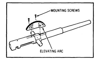
**Step 3:** Remove the elevating arc from the barrel by removing the two mounting screws
