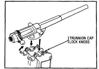
**Step 6:** Open the trunnion caps. Remove the barrel from the chest and attach it to the mount assembly by placing the trunnions in the recesses. Lock the trunnion caps.
