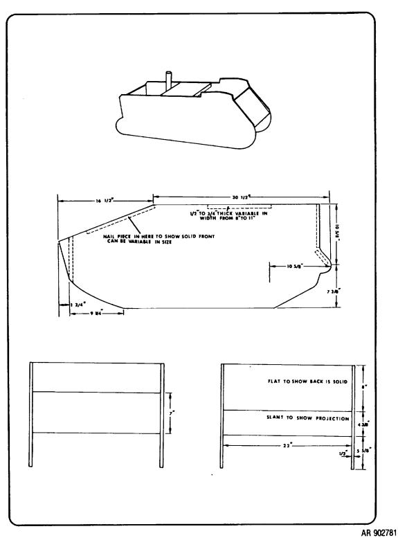
Figure 2-10. Armored personnel carrier target model
