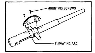
**Step 8:** Remove the elevating arc from the gun barrel by removing the two mounting screw.
