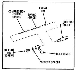
**Step 3:** Replace the spring and/or firing pin as required, then reassemble parts in reverse order.
