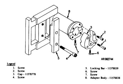
Figure 4-5. Disassembly/assembly of adapter assembly PN 11578865 for M101A1
