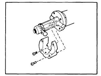
**Step 6**: Lock the barrel into position by securing the adapter cap to the body Do not tighten the four screws yet.
