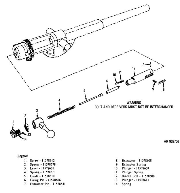
Figure 6-1. Disassembly/assembly of breech bolt assembly
