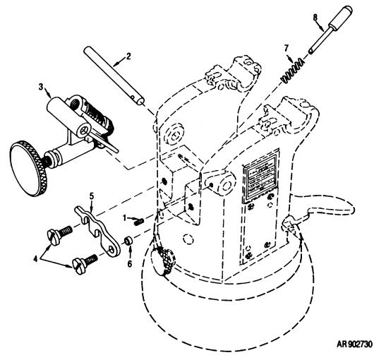
Figure C-8. Mount assembly - partial exploded view
