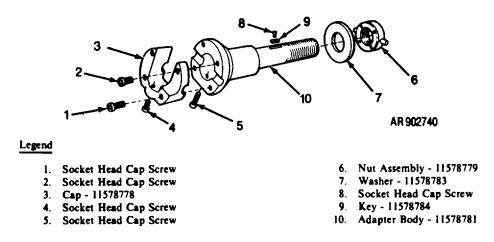
Figure 4-8. Disassembly/assembly of adapter assembly PN 11578780 for M109 series and M107/M110
