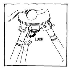
**Step 2:** With the rear leg pointing opposite to the direction of fire, spread the two front legs about 4-1/2 feet apart and lock them in place by turning the leg locking levers to the outward position.
