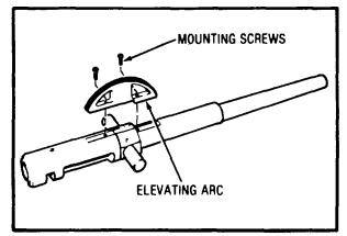
**Step 3:** Remove the elevating arc from the gun barrel by removing the two mounting screws.
