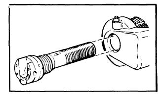
Step 5: Insert the adapter (top up) in the breech-block.
