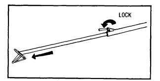
**Step 3:** Unlock the locking lever at the bottom of the rear leg and extend the leg about 15 inches. Lock it in the extended position by tightening the lower locking lever. Then place the rear leg in the ground so the top of the tripod assembly is approximately level.
