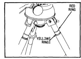
**Step 4:** Extend each leg until the yellow ring can be seen. The yellow ring indicates the center of the threads. There are two red rings on each leg which indicates that the rotating collar has reached the end of the threads. Do not turn the rotating collar beyond the red rings.
