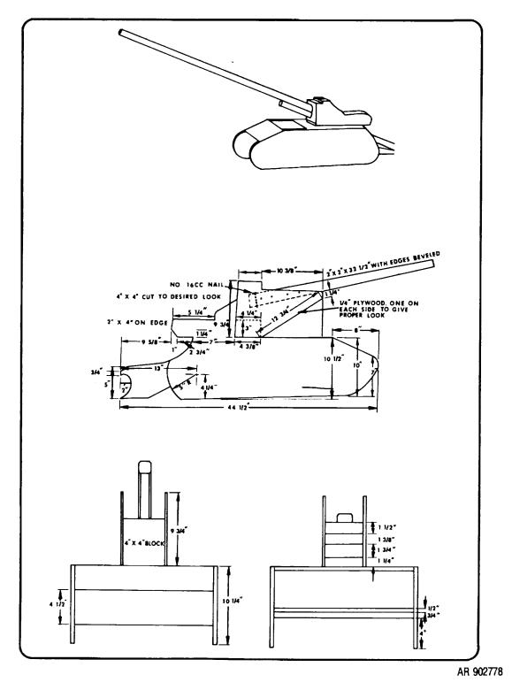
Figure 2-7. 175-mm Gun target model
