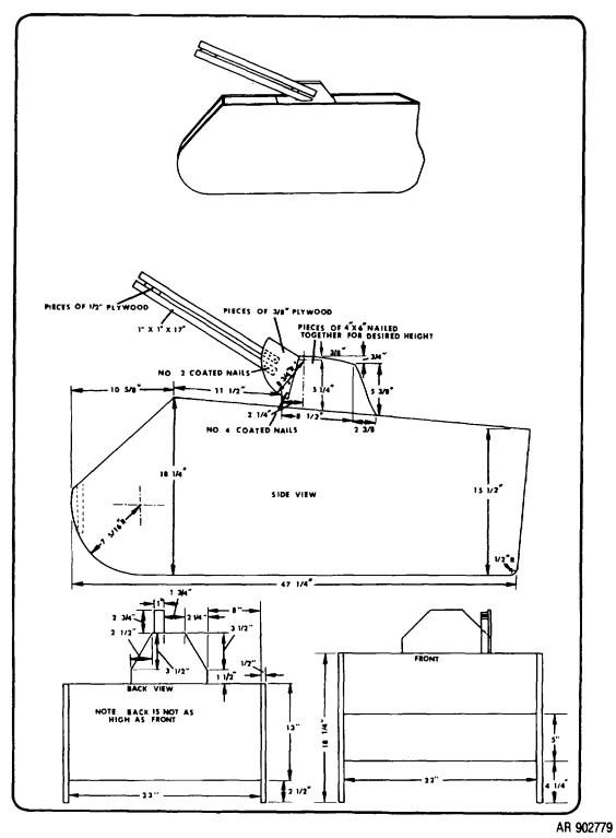
Figure 2-8. Self-propelled antiaircraft vehicle target model
