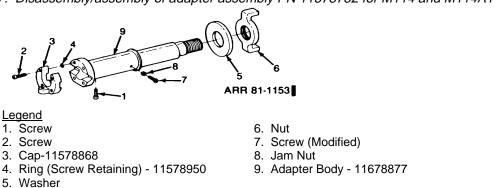
Figure 4-7A. Disassembly/assembly of adapter assembly PN 11578876 for M114A1 Change 1 4-7
