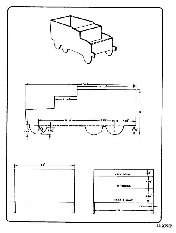
Figure 2-11. 2 1/2 Ton target model
