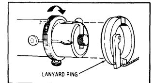
**Step 8:** Turn the safety ring to the "tire" position. Place the lanyard ring over the rear of the breech, matching the openings of breech and the lanyard ring.
