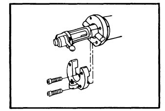
**Step 9:** Lock the barrel into position by securing adapter cap to the body. Do not tighten the four screws yet.
