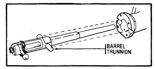
**Step 10:** Place the gun barrel in the adapter and engage the barrel trunnions with the adapter slots.
