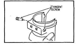
**Step 4:** Sight the tube onto a distant aiming point (1, 500 meters). Aline panoramic telescope sight on the same distant aiming point using the tangent screws on the telescope mount or the telescope boresight adjusting screw
