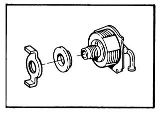
**Step 4:** Aline pin on adapter with slot in washer and install washer. Install nut and tighten completely.
