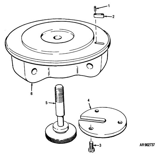
Figure C-15. Tripod base assembly - exploded view
