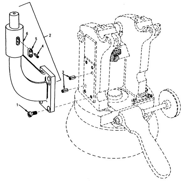
DRILL EXISTING HOLES TO 0.196 + 0.002 DIAMETER AND 0.63 + 0.02 DEEP TO ACCEPT SPRING PIN (3) DRILL EXISTING HOLES TO 0.118 + 0.004 DIAMETER AND 0.41 + 0.01 DEEP TO ACCEPT SPRING PINS (4)
