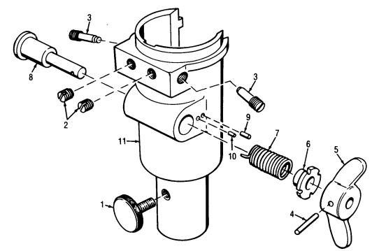
ASSEMBLE SPRING (7) AND RETAINER (6) FOR A MINIMUM OF 2 IN-LB TORQUE WITH THE WINGS OF HANDLE (5) TURNED 45 DEGREES FROM VERTICAL
