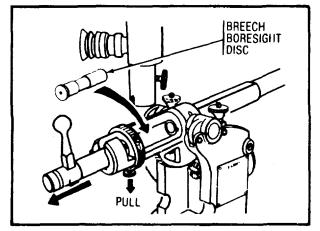
**Step 2:** Remove the bolt. Install breech boresight disc. (The breech boresight disc is a fired cartridge case that has a 1/16-inch hole drilled in the center of the cartridge base.
