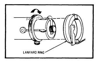
**Step 11:** Turn the safety ring to the :fire: position. Place the lanyard ring over the rear of the breech, matching the openings of breech and the lanyard ring.
