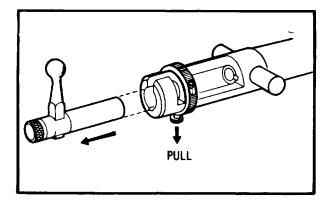
**Step 1:** Remove the bolt by pulling down on the bolt locking cap and pulling bolt to the rear.
