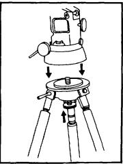
**Step 5:** remove the mount assembly from the storage chest and place it on top of the tripod assembly. Aline key on tripod base with keyway in bottom of mount. Then tighten the mount locking screw into the mount assembly.
