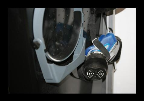
Pegboard on the legs of the bench keeps the larger items like the respirator or visor from clogging the main work area but are within reach.
